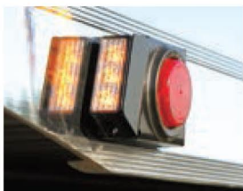
Side-mounting helps to minimize potential blockage from payloads
