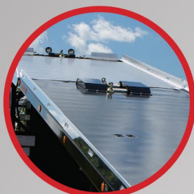
LOW PROFILE WINCH SYSTEM ALLOWS FLAT ALIGNMENT OF UPPER AND LOWER DECK
