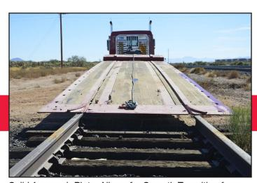
Solid Approach Plate Allows for Smooth Transition from Rail to Trailer without Heavy Ramps or Drop-in-Rails
