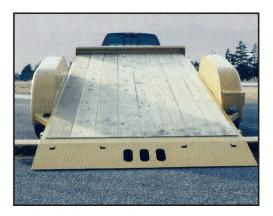
A full width rear light bar for added safety protection with machined safety approach plate.
