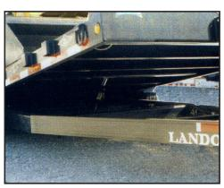
The Landoll tilt control system and the 2½" x 16" cushion cylinder can hold the deck in a tilted position or smoothly return the deck to transport position.
