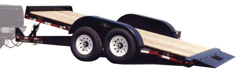
A 6"channel iron frame under the main frame for superior strength. A solid formed 6" height headboard for protection. (Stake pockets shown for optional removable sideboards)
