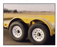
14-gauge molded fenders and anti-slip steps for strength and safety.
