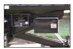
**Hydraulic Control Box**A well-protected, illuminated hydraulic control box is located just rear of the axle.
