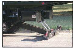
**Standard Stabilizer Bar**The heavy-duty stabilizer bar also serves as a dock level hydraulic lift that raises the bed to a maximum of 59" with 30,000 lb. capacity.
