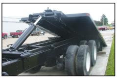
**Hydraulic System**The Loadoll III uses welded hydraulic cylinders with chrome plated rods for long trouble-free service.
