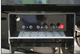
**Dual Hydraulic Controls** Well protected, illuminated hydraulic controls are located just rear of the axle.
