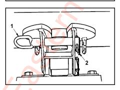
Install the retaining bolts thru the keeper bracket and into the adapter. Using a wrench, tighten the retaining bolts until snug.
