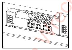
Using the winch control levers, unwind some wire rope from the winches to relieve the pressure on the winch free-spool device
