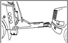
The recovery vehicle's position should be approximately nine (9) feet from the casualty vehicle. Reposition the recovery vehicle if necessary.
