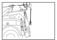
Position the boom head by using the boom up, down, in and out levers as necessary.
