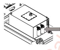
Lube Point(s) – Replaceable Elements Interval – Change every 250 hours or Semi Annually Or as indicated by condition indicator gauges
