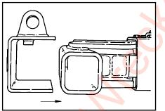
1. Slide the 5th wheel plate adapter onto the crossbar pivot of the underlift. The 5th wheel adapter plate is stored in the toolbox.
