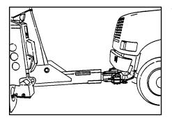
10. Raise the casualty vehicle into towing position observing the far end for sufficient ground clearance.
