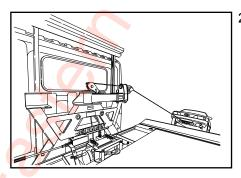
21. Attach the wire rope/cable to the vehicle to be pulled. Always use V-straps or hook-up chains to attach the wire rope/cable to the vehicle. Refer to the AAA or vehicle manufacturer's towing manual for correct attachment points. A snatch block may be used if required to pull from a lower angle. (See snatch block operation)
