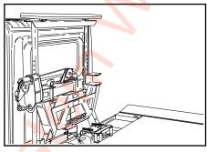
7. The recovery boom can pivot easily from the left side to the right side or right side to the left side of the vehicle. To pivot the recovery boom, remove the retaining pin.
