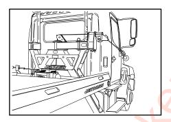
20. Next, unreel enough of the wire rope/cable from the winch to make your hookup. This can be done by depressing and holding the winch control button on the hand controller and unreeling the wire rope/cable from the winch while keeping the wire rope/cable taut. You can also use the remote winch free spool device. This allows for rapid unspooling of the wire rope/cable from the winch. (See winch operation)
