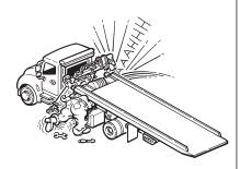
Block up the deck before performing any service or maintenance work under the deck.
