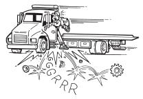
Don't travel with the PTO engaged. Damage to the recovery vehicle's transmission and hydraulic components will occur. Engage it only while operating the controls.
