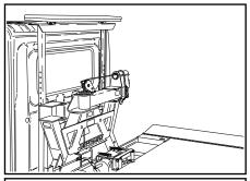
Pivot the recovery boom to the other side of the recovery vehicle.
