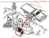
Know the loads being moved. DO NOT OVERLOAD! NEVER exceed the rated capacity of the body or truck chassis and it's components.
