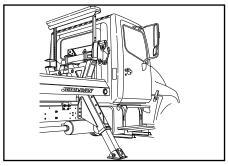
12. The left and right stabilizers operate independently of each other. The stabilizers only need to touch the ground to support the load. Do not attempt to use the stabilizers to level or raise the truck.
