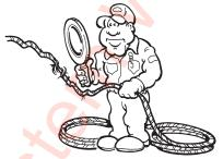
Maintain winch cable/wire rope in good condition. Replace when worn, kinked or frayed. Do not use cable clamps.
