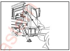
26. Unhook the wire rope/cable from the recovered vehicle.
