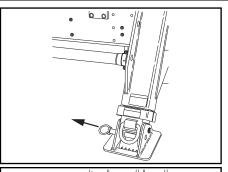
Remove the spade retaining pin allowing the integral spade to drop down.
