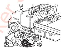
Don't operate the engine faster than recommended. Excessive speeds can damage PTO, hydraulic pumps, and winches.
