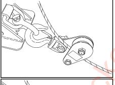
8. Place the wire rope/cable across the sheave.
