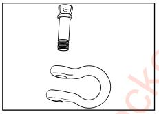
2. Align the hole in the shackle with a hole in the tie back plate or over the "D" Ring.
