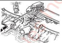
Vehicle must be located on a firm surface that will provide support for the stabilizer loading. Use caution when setting up near overhanging banks or excavations.
