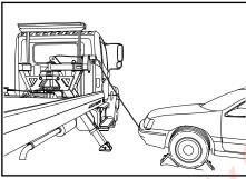
24. Secure the recovered vehicle to prevent it from rolling. Place wheel chock against the tires.
