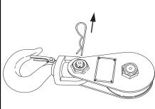
4. Remove the sheave side plate screw pin cotter pin.
