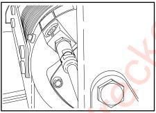
Visually verify that the free spool knob is locked in the free spool position. The winch clutch is now locked out and the wire rope/cable may be pulled off by hand.
