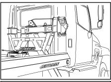
27. Reel in any extra wire rope/cable and secure.
