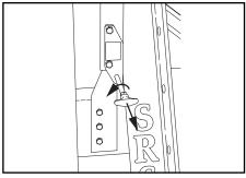
To disengage the winch "free-spool", pull out on the "T" handle and turn the handle 90°. The handle should remain in the "free-spool" position Never pull the free spool knob while the wire rope/cable is under load.
