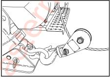
10. Reinstall the sheave plate screw pin and cotter.
