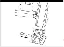
17. Re-insert the spade retaining pin.
