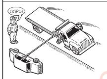
Always lower the stabilizers before pulling a load to stabilize the truck.
