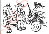
Never make a lift or pull with the cable attached to light gauge or sheet metal parts; use the frame or major structural members.
