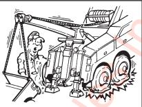
Avoid using the boom raise or boom up control to lift a load. This causes undue stress and weight loading on the rear axle. Use the winch to lift the load.
