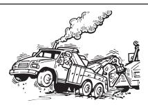
Don't expect your wrecker to tow loads equal to the wrecker ratings. Wrecker ratings apply to loads imposed during recovery with the wrecker properly stabilized.
