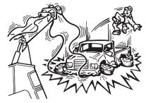
Don't disengage the winch drum clutch while the wire rope is loaded.
