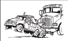
Don't tow a vehicle that reduces the weight on the front wheels of the wrecker more than 50 percent. (SAE J2512)
