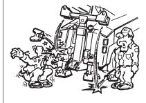
Never fold the boom up into storage position without removing the towing adapters.
