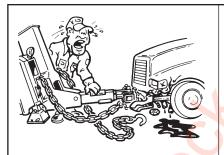
Never attach the chain hooks in such a way as to damage brake lines or other functional parts.
