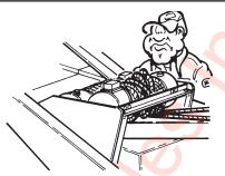
Never allow the wire rope to cross wrap (criss-cross) on the winch drum. Crushing of the wire rope can cause premature wire rope failure.
