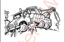
Never tie down the front end of your wrecker for recovery work of heavy lifts. You will likely damage the truck frame if you do.
