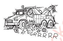
Don't travel with the PTO engaged. Damage to the recovery vehicle's transmission and hydraulic components will occur. Engage it only while operating the controls.
