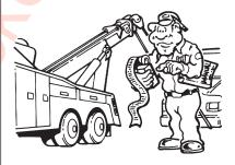
Be sure of your lift or pull and do not exceed the working limit of the wire rope or hook. Rig to keep the estimated amount of pull well within equipment ratings. Use wire rope breaking strength ratings only for selecting replacement wire rope.
