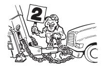
Always use two safety chains and two tie-down chains when towing all vehicles, regardless of distance.
