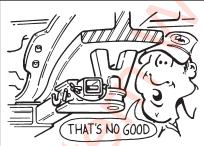
Don't use towing forks that are not of proper size for the pickup requirements.
