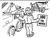
Jog the winch control lever to be sure of complete engagement of the clutch gears before making a lift or pull.
