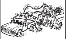
After rigging wire ropes, don't begin pulling without rechecking connections. Make sure that all wire ropes and snatch blocks are securely attached and cannot accidently pull loose.
