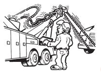
Never completely unwind wire rope from a winch while loaded. Always be sure that a minimum of five (5) wraps of wire rope are on the drum at all times. (SAE J706)
