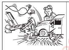
You should never make a lift or movement while close to or under the vehicle being lifted!
