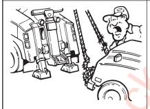
Never wrap the wire rope around frames or cross members. Use chains and hook the wire rope to the chains.
