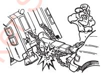
Check that the chain does not become over tensioned when raising the towed vehicle to the towing position or during the towing operation.
