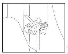
1. Remove the retaining bolts and wing nuts or pad locks, which ever your unit may have.
