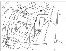
15. Close the dolly retaining latch by pushing the top away from you.
