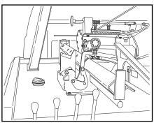
11. The axle cross tube rails need to be stored with the wheel ramp plates turned in and up.
