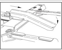
Hook the loading ramp onto the wheel grid and engage the rear hooks on the back side of the grid.
