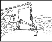
21. Retract the boom slowly drawing the vehicle forward until the stand offs are fully retracted and the "CAM" handles retract to the closed position for traveling.
