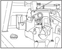
Remove the dolly wheel assemblies, the axle cross tube rails and the pry bar/jack bar.
