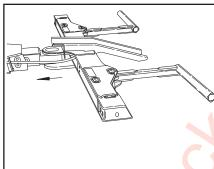
Completely retract the wheel grid for loading.
