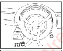
With the vehicle lifted just barely off the ground, insert the end of the strap through the sewn loop on the other end of the strap to form a loop. Put the loop over the tire as shown with the strap resting on the tire at the ten o'clock and two o'clock positions.
