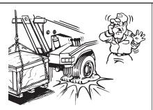
Avoid using the boom raise or boom up control to lift a load. This causes undue stress and weight loading on the rear axle.
