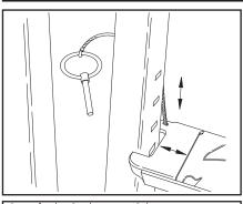
Adjust the upper and lower tire stops so that they will contact and restrain the front tire when loaded.
