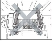
11. With the wire rope tight, slowly wind it in, observing both the work and the drum. Be sure the wire rope strands do not cross wrap or criss-cross on the drum. Observe the path the work must travel for snags or obstructions which could stall the movement and overload the wire rope.
