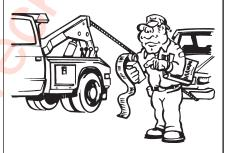
Be sure of your lift or pull and do not exceed the working strength of the wire rope or hook. Rig to keep the estimated amount of pull well within equipment ratings. Use wire rope breaking strength ratings only for selecting replacement wire rope.
