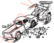
Don't tow a vehicle on its drive wheels unless steps have been taken to protect its transmission and differential. Follow the recommendations of the vehicle manu-facturer. As an alternative, use a towing dolly.
