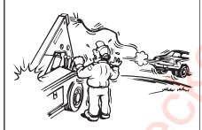
Never completely unwind wire rope from a winch while loaded. Always be sure that a minimum of five (5) wraps of wire rope are on the drum at all times.
