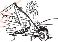
Never make a lift or pull with the wire rope attached to light gauge or sheet metal parts; use the frame or major structural members.
