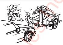
All boom placement functions should be made with the winch wire ropes set in "free spool" to avoid over tensioning or breaking the winch wire ropes.
