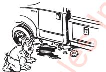
Don't operate the wrecker's engine faster than recommended. Excessive speeds can damage PTO, hydraulic pumps, and winches.
