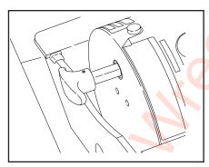
Reengage the winch "free-spool" by turning the handle back 90°.
