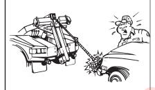
Never wrap the wire rope around frames or cross members. Use chains and hook the wire rope to the chains.
