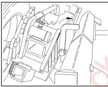
15. Close the dolly retaining latch by pushing the top away from you.
