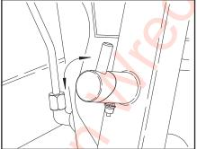
25. Rotate the "CAM" handles on the hold back bars 180° to the open position.
