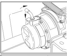
10. Re-engage the winch drive by pushing down on the spring steel latch plate and turning the handle 180°. Confirm winch engagement by jogging the winch control. Now slowly take up the slack in the wire rope.
