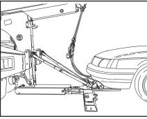
13. Maneuver the sling under the vehicle to be towed, far enough under so the vehicle will ride on the rubber belts.
