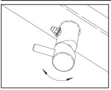
20. Rotate the "CAM" handles on the hold back bars 180° to the closed position.
