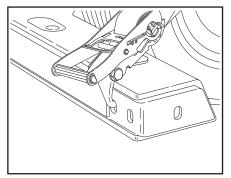
Place the hook of the ratchet into one of the holes on the front side of the grid. Again, try to use the hole that is closest to the tire.
