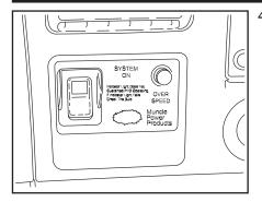
4. Engage the Power-Take-Off (PTO) or Clutch Pump and the hand controller using the "Control" switch in the switch panel. Most trucks will automatically throttle up when the parking brake is set and the transmission is park or neutral. NEVER TRAVEL WITH THE POWER-TAKE-OFF or CLUTCH PUMP CONTROL ENGAGED. This could result in damage to the PTO or Clutch Pump unit and the truck transmission.
