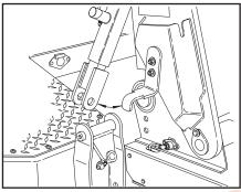
27. Swing the hold back bars in toward the tow sling storage brackets on the side of the boom. Allow the hold back bars to retract as necessary.
