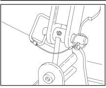
26. Remove the pins from the hold back bars at the rear of the body.
