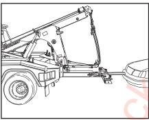
10. Carefully extend and lower the wrecker boom to allow the tow sling head to rotate outward and down away from boom.
