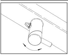
Rotate the "CAM" handles on the hold back bars 180° to the open position.
