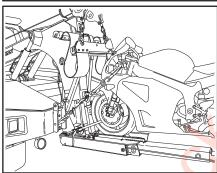
16. Place the hook on one end of the "front" strap to the loop of the lasso strap on the handle bars and place the hook on the other end to the rear of the wrecker body and tighten with the ratchet. Repeat for the other side.
