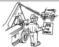
Jog the winch control lever to be sure of complete engagement of the clutch gears before making a lift or pull.
