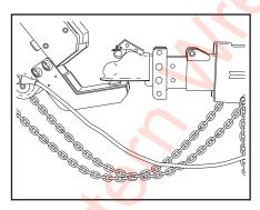
6. Connect the trailer lights and attach safety chains.
