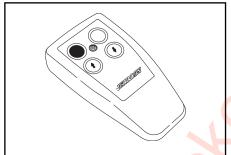
3. To turn off the power to the hand controller, simply press the red button. The red light will stop illuminating.
