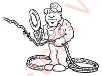
Maintain winch cable/wire rope in good condition. Replace when worn, kinked or frayed. Do not use cable clamps.
