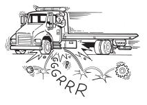
NEVER travel with the PTO engaged. Damage to the recovery vehicle's transmission and hydraulic components will occur. Engage the PTO only when operating the controls.
