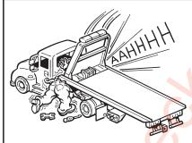
Block up the deck before performing any service or maintenance work under the deck.
