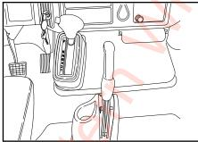
Place the carrier's transmission gear selector into Neutral or Park and set the parking brakes.
