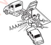
NEVER winch from the side of the bed. Winch only from the rear with load centered and in line with the winch. Failure to do so can result in winch or wire rope damage and/or bodily injury. NEVER USE THE DECK WINCH FOR SIDE PULLING.
