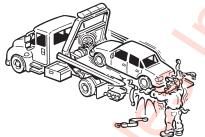
NEVER work behind the truck with a vehicle on the deck unless the vehicle is secured at the front of the deck. (Do not rely on the winch to hold the load).
