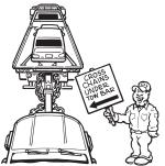
Use separate safety chains from the towed vehicle to the subframe for standard towbar and wheel
