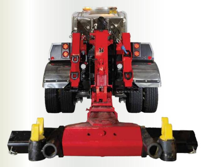
Every model of Zacklift can be removable FIFTHWHEELER mounted or Permanently Mounted
