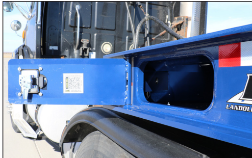
Standard Upper Deck or Side Opening Toolboxes. Both with Stainless Steel Bottom and LED Lights Inside.
