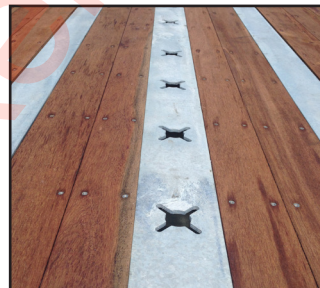
Center Deck Keyhole Tie Downs Flush with Wood
