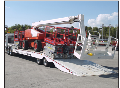
No Flip Tail Means You Can Utilize The Whole Deck
