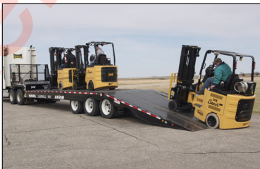
15' Ramp Delivers 11° Degree Load Angle
