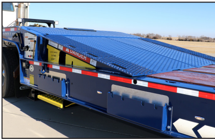
Upper Deck Air Ramp Features An 11° Load Angle and Low Clearance
