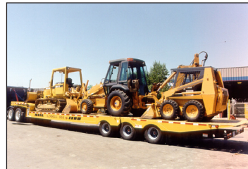
The Undercarriage is Behind the Hinge in Travel Position So You Can Load the Entire Deck
