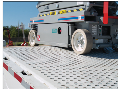
Upper Deck Air Ramp Features An 11° Load Angle and Low Clearance
