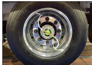
Wheel Options: Crossfire Air Equalizers or Meritor Tire Inflation System; Optional Disc Brakes
