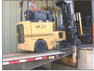
The Tail Can Lift an Impressive 24,000 lbs. To Dock Height 53"
