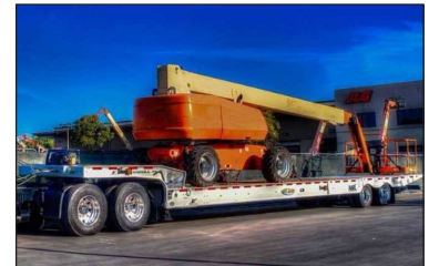
The Undercarriage is Behind the Hinge in Travel Position So You Can Load the Entire Deck
