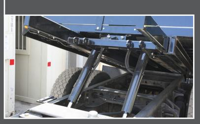
Hydraulic System The Loadoll II uses welded hydraulic cylinders with chrome plated rods for long trouble-free service.
